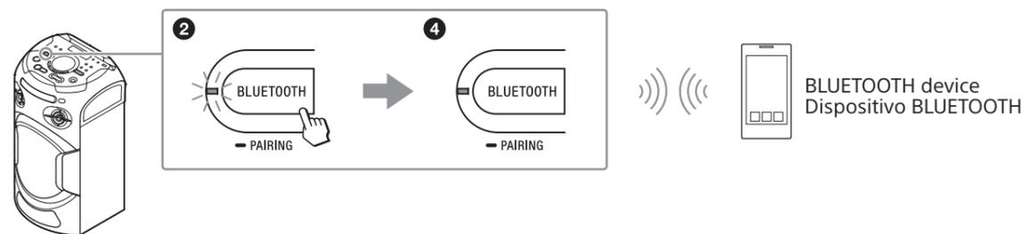
Be sure to place the BLUETOOTH device within 1 meter from the unit.
