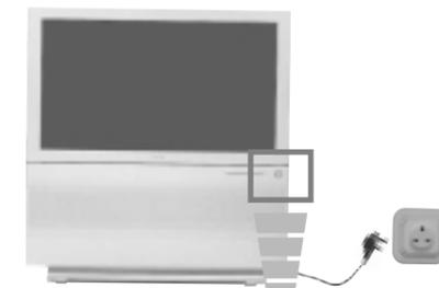
Connect the TV plug to the mains socket (220-240V AC, 50Hz).
