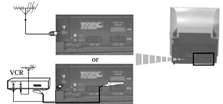
① The Scart lead is optional. If you use this optional connection it can improve the picture and sound quality when using a VCR.
