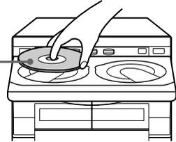
To insert a third disc, press DISC SKIP/ EX-CHANGE to rotate the disc tray.
