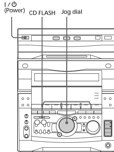
➔ Press and hold CD FLASH during playback at the point you want to start the Flash function, and release to resume normal play.
