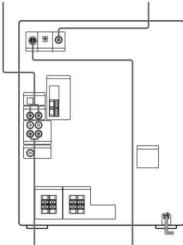
To the audio inputs of the VCR using an optional audio cable
