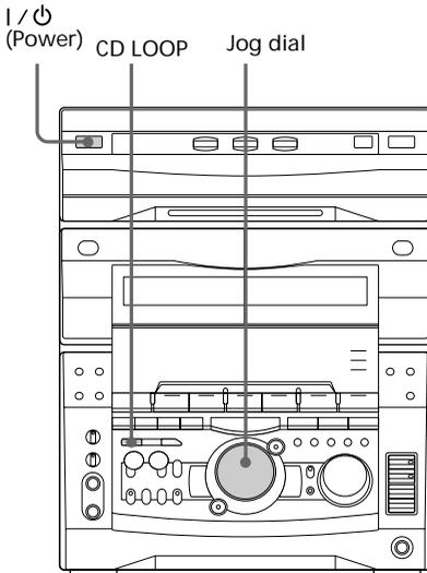
➔ Press and hold CD LOOP during playback at the point you want to start the Loop function, and release to resume normal play.
