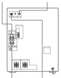
To the audio inputs of the VCR using an optional audio cable
